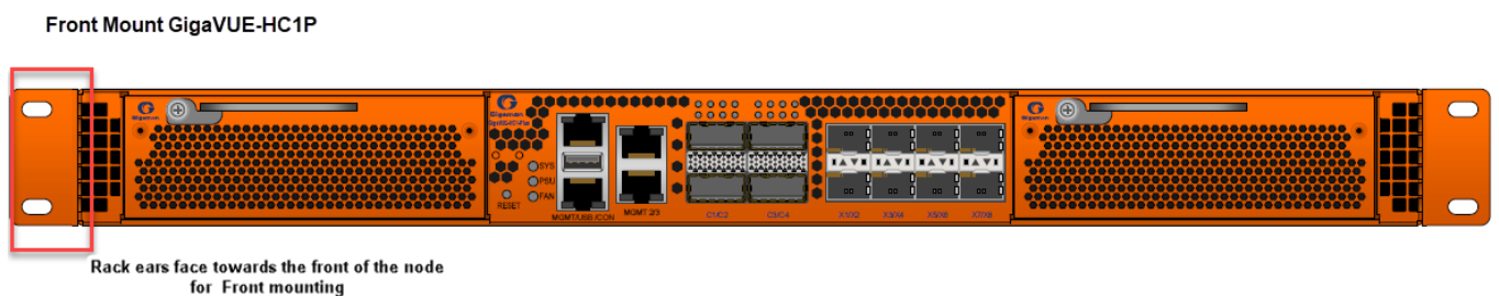
Figure 4 Rack Ears for Front Mount (Reverse Rack Ears for Center Mount)
